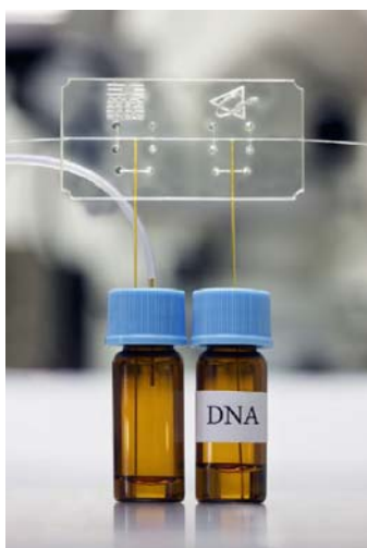
Fig. 3 Fabricated lab-on-a-chip component with integrated MOF. The MOF is optically connected to input/output optical fibers (coming from left and right). Fluid samples are injected into the MOF through silica capillary tubes
